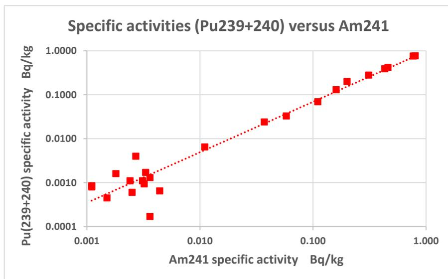
**Fig. 1.** The specific activity (i.e. concentration) of Pu(239+240) is plotted against that of Am(241) on logarithmic scales. The data in the lower decades has a wider spread, as expected as the limits of detection approach. However, the it is still consistent with the trend in the highest decades.
